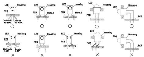
$^{\prime}\bigcirc$  " Correct mounting method "imes" Incorrect mounting method
