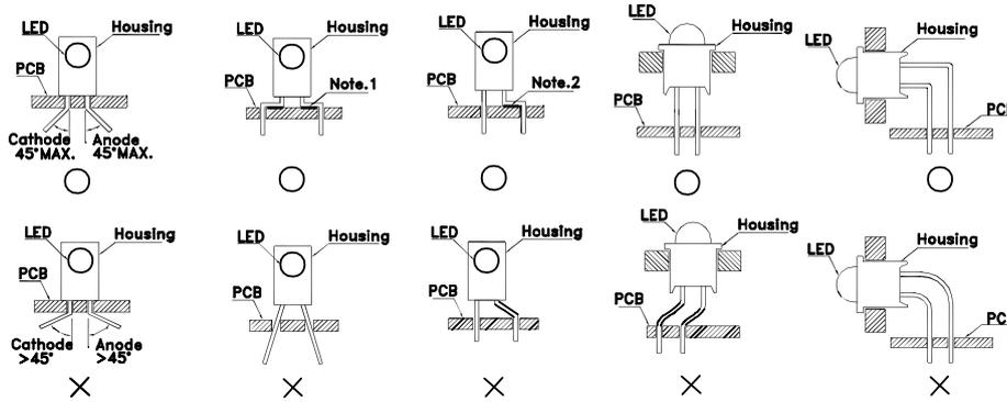
"O" Correct mounting method "X" Incorrect mounting method
