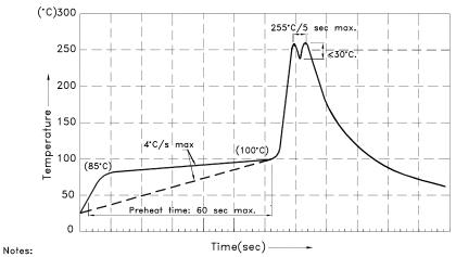
1.Recommend pre—heat temperature of 105°C or less (as measured with a thermocouple attached to the LED pins) prior to immersion in the solder wave with a maximum solder bath temperature of 260°C
