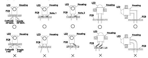
" $\bigcirc$ " Correct mounting method " $\times$ " Incorrect mounting method
