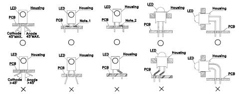
"Correct mounting method "X" Incorrect mounting method
